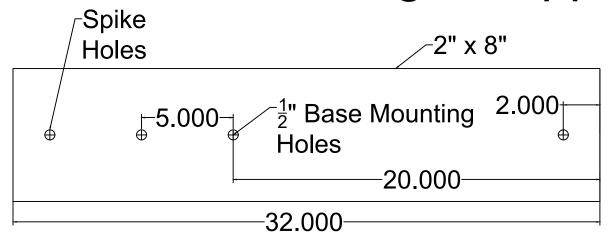
Wood base for our double popper bases using 32" of 2x8. The hole spacing of base mounting holes are the only critical measurements to get right. The spike holes and the overall dimension can very depending on what you want and have available. Bumper is optional, but sometimes needed.
